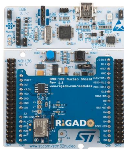
Figure 1: BMD-100 Nucleo Shield installed on a STM32 Nucleo board
