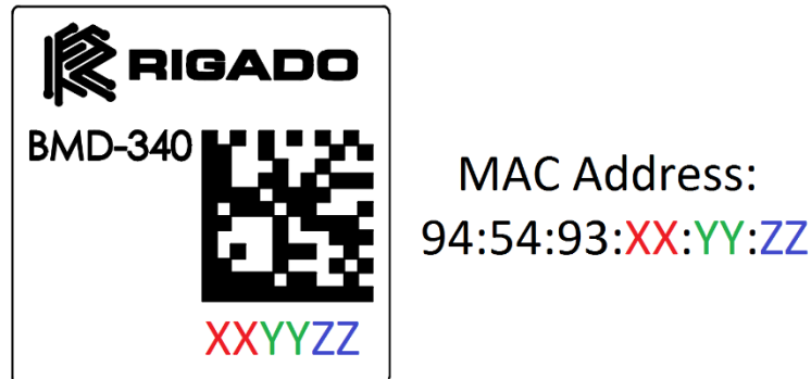
Figure 11 – BMD-340 MAC Address on Label
