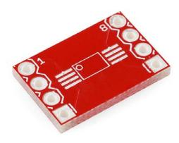
**Description:** 8-Pin SSOP to DIP break out board. The footprint was rotated to accommodate different width SSOP devices and can be used with 8 pin SSOPs. Designed to be used with 0.65mm pitch devices but can also be used with 0.025" pitch devices (comes out to  $\sim$ 0.635mm). We've made these 0.635mm devices fit just fine. Can be used with packages from 0.200" (5mm) up to 0.450" (11.4mm) in width.
