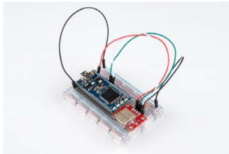
USB Type A Female Breakout added to the mbed LPC1768
