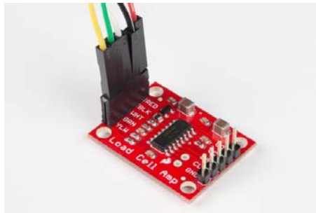
Load cell wires hooked up to the HX711 Amplifier board
