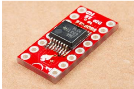
14 pins in a 16-pin adapter.
