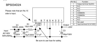
For acutual usage, Please kindly evaluate and confirm our part mounted in your product, Especially, Please make sure to confirm whether the load current exceed Max. rated current by using the current probe.
