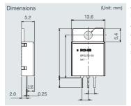
All necessary components are integrated into the TO-220 package. And no input or output capacitors are required. The result is a mounting area 6 times smaller than conventional solutions. In addition, the units are pin-compatible with the 3-terminal LDOs, making replacement easy.
