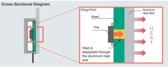
Heat dissipation is required, even for surface mount DC/DC converter ICs. The BP5275 series was specially designed for optimum heat dissipation in a compact form factor, minimizing mounting area.
