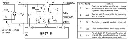
Please verify operation and characteristics in the customer's circuit before actual usage. Ensure that the load current does not exceed the maximum rating.
