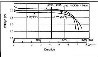
High temperature discharge under 150 k $\Omega$  (equivalent to approx. 20 $\mu$ A)
