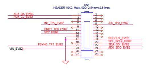
To connect to the Discovery Board you will need to connect these 5 pins on the Invensense EVB. Most Invensense EVBs do not populate the pins 1-4 and 25-28.
