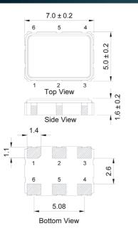
PAD FUNCTION: 1: ENABLE CONTROL or NC 2: ENABLE CONTROL or NC 3: GND 4: OUT 5: OUTN 6: VDD
