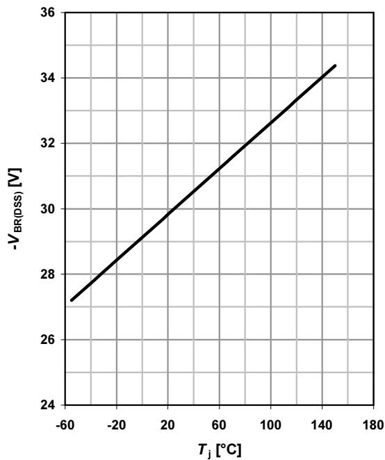
**28 Drain-source breakdown voltage (N)**
