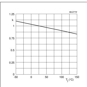
$$k = \frac{V_{GS(th)} \text{ at } T_j}{V_{GS(th)} \text{ at } 25 \text{ }^{\circ}\text{C}}$$
