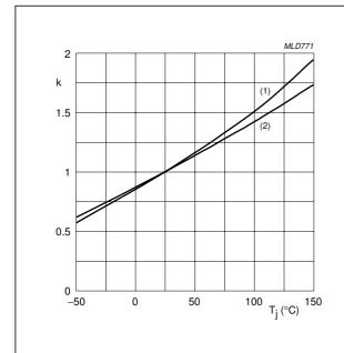
$$k = \frac{R_{DS(on)} at T_j}{R_{DS(on)} at 25 °C}$$
