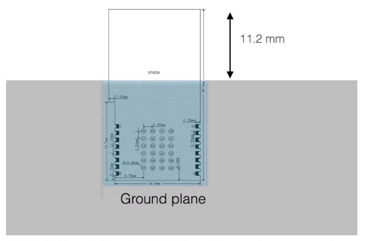
1.BT832X module extends 11.2 mm from edge or ground plane of the host PCB board
