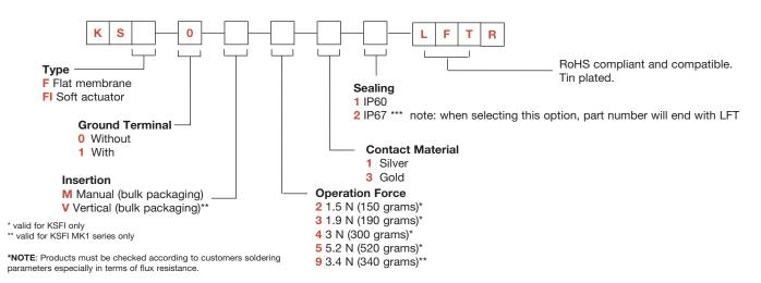
Overload resistance: 40N, 1 time Sealing: IP60 or IP67
