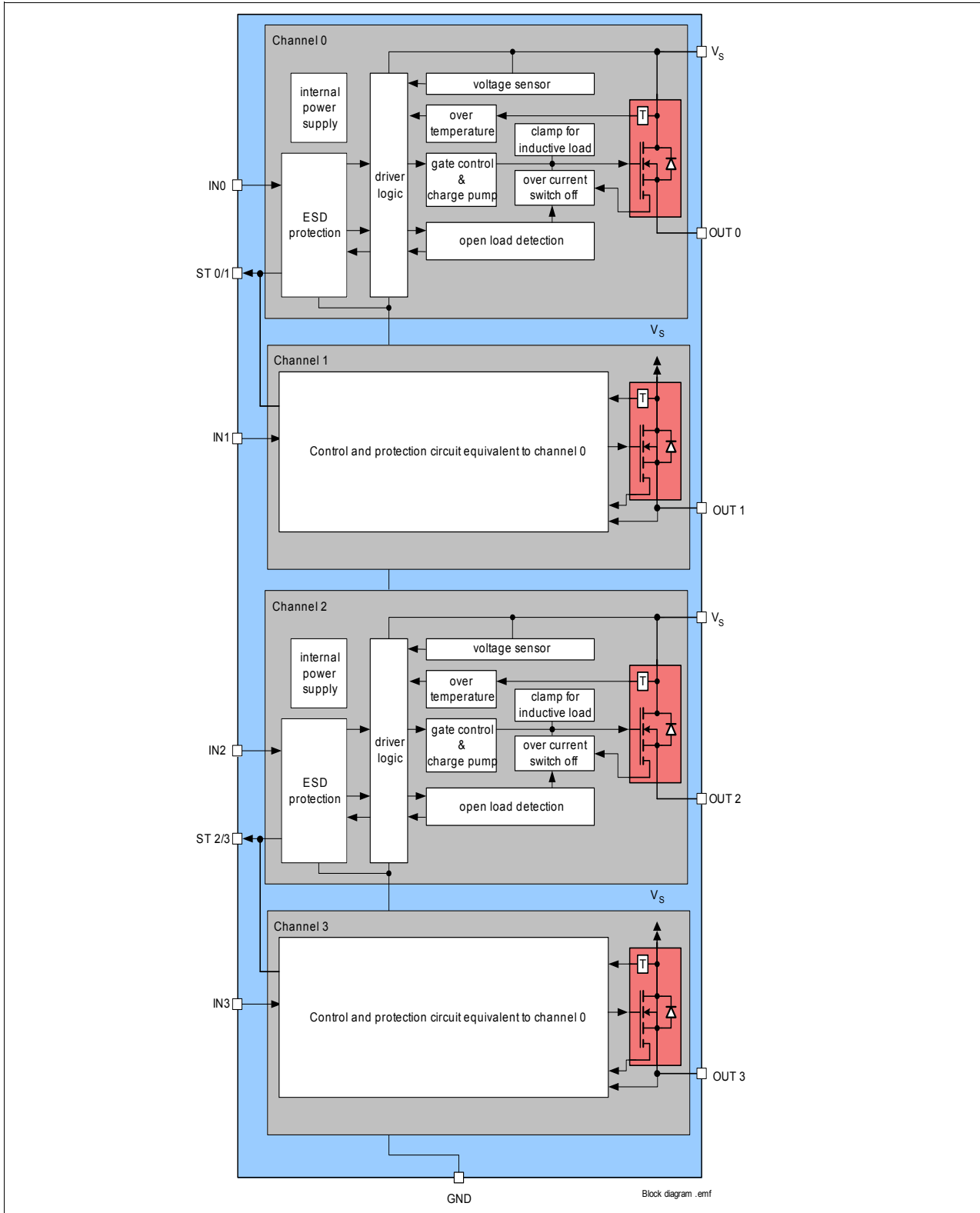
Figure 1 Block diagram for the BTS4130QGA
