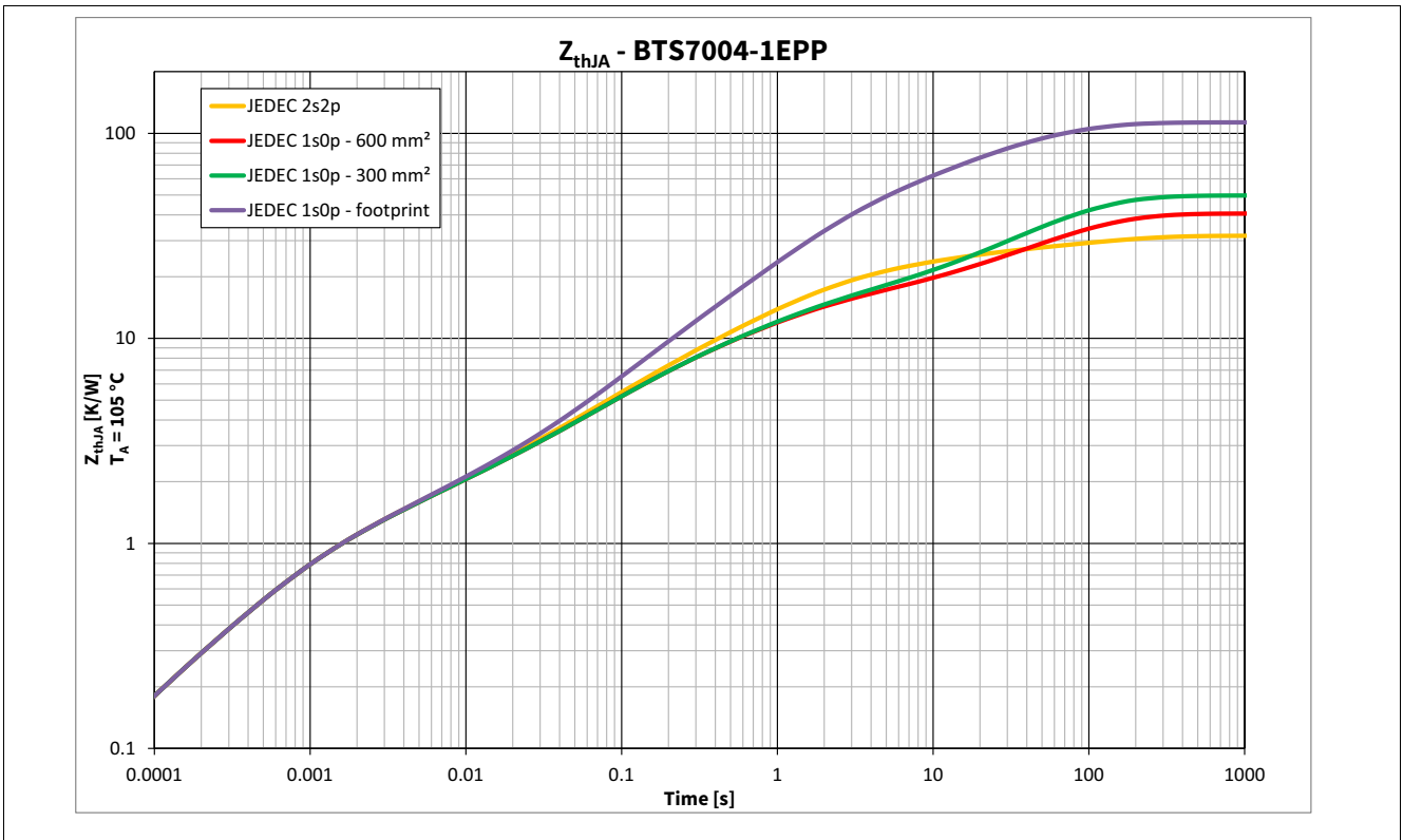
Figure 9 Typical Thermal Impedance. PCB setup according Chapter 4.4.1
