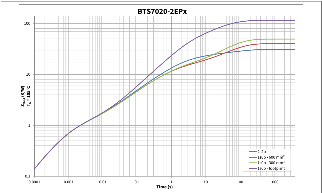
Figure 9 Typical Thermal Impedance. PCB setup according Chapter 4.4.1
