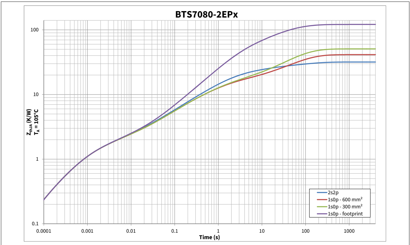
Figure 9 Typical Thermal Impedance. PCB setup according Chapter 4.4.1
