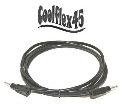
Coolflex45 cables get their name from the extremely low temperature rise under high current conditions. Testing under a continuous AC load of 45 Amps resulted in only a 30°F (17°C) temperature rise. Coolflex45 cables were also exposed to overcurrent loads of 70 Amps for fifteen seconds and resulted in only a 14°F (8°C) temperature rise. (Note, all testing was performed by an independent, certified laboratory)
