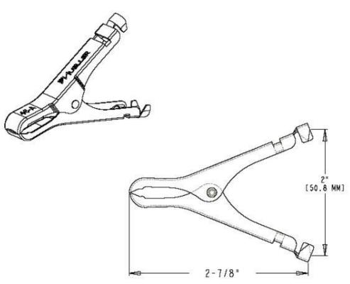
Dimensions: Length: 2.88" (73 mm); Width: .48" (12 mm); Height: 2" (51 mm) Jaw opens to: 1.13" (29 mm)
