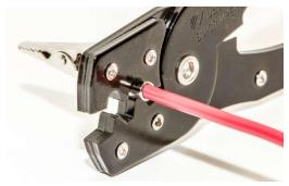
3) Important! Align the clip such that the "tooth" of the crimper faces the bottom of the clip.
