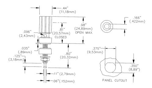
Mounts in Panels between .070" and .250" (1.77-6.35) Thick Accepts Standard 4mm Banana plugs or bare wire or spade lugs
