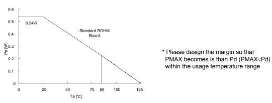
Figure 83. SSOP5 Power dissipation heat reduction characteristics (Reference)
