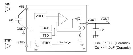
Figure 2. Block Diagrams
