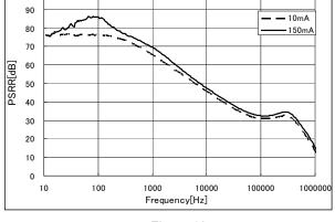
POWER-SUPPLY RIPPLE REJECTION vs FREQUENCY
