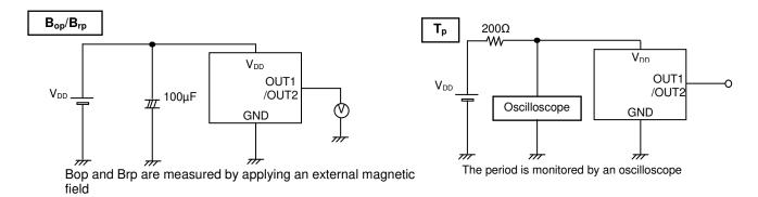
Figure 1. Bop, Brp Measurement Circuit
