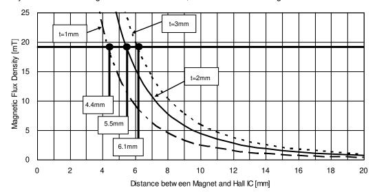
Figure 18. Magnetic Flux Density vs Distance between Magnet and Hall IC
