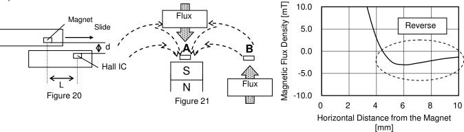
Figure 22. Magnetic Flux Density vs Horizontal Distance from the Magnet
