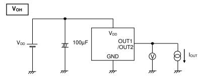
Figure 3. V<sub>OH</sub> Measurement Circuit
