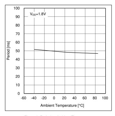
Figure 8. Period vs Ambient Temperature
