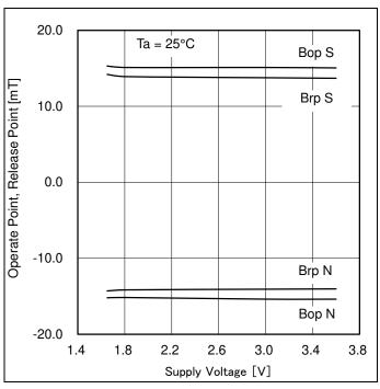
Figure 7. Operate Point, Release Point vs Supply Voltage
