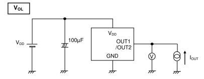
Figure 4. Vol Measurement Circuit
