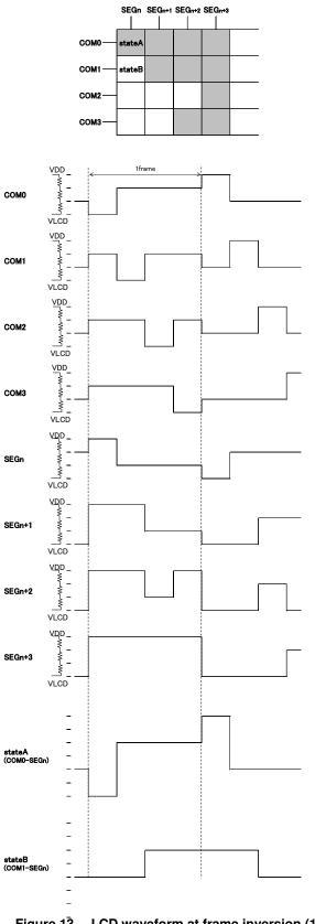
Figure 13. LCD waveform at frame inversion (1/3bias)
