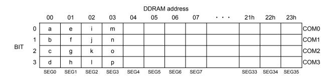
Data transference to DDRAM will be executed in every 4bit data. So it will be finished to transfer with no need to wait ACK.
