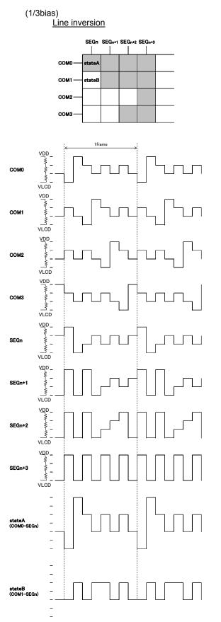
Figure 12. LCD waveform at line inversion (1/3bias)
