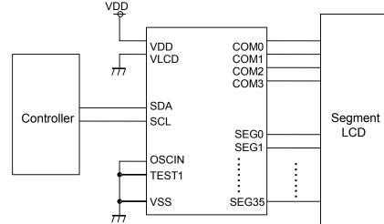
Using internal oscillator
