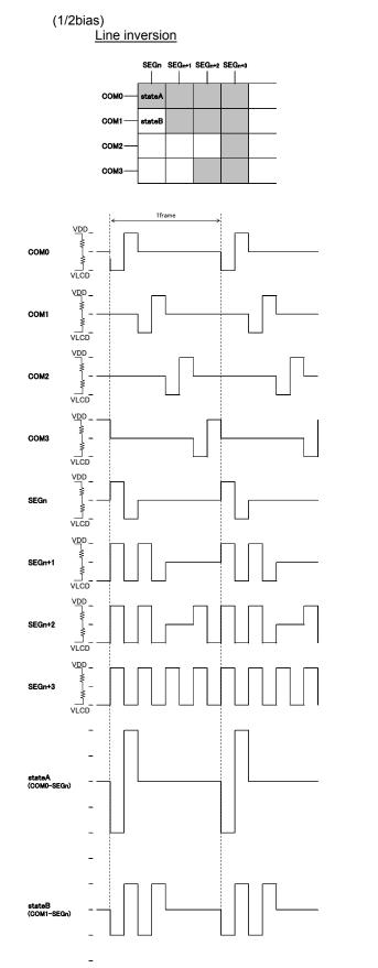
Figure 14. LCD waveform in line inversion (1/2bias)
