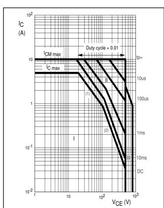
Fig. 15. Forward bias safe operating area.  $T_{hs} \le 25 \, ^{\circ}C$
