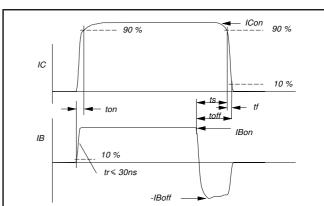
Fig.4. Switching times waveforms with resistive load.
