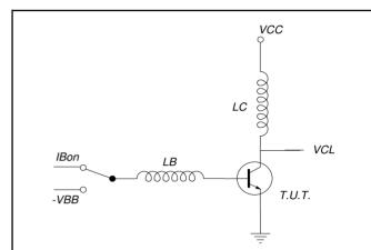
Fig.14. Test Circuit for reverse bias safe operating area  $V_{cl} \leq 1000V; \ V_{cc} = 150V; \ V_{BB} = -5V; L_B = 1\mu H; \ L_c = 200\mu H$
