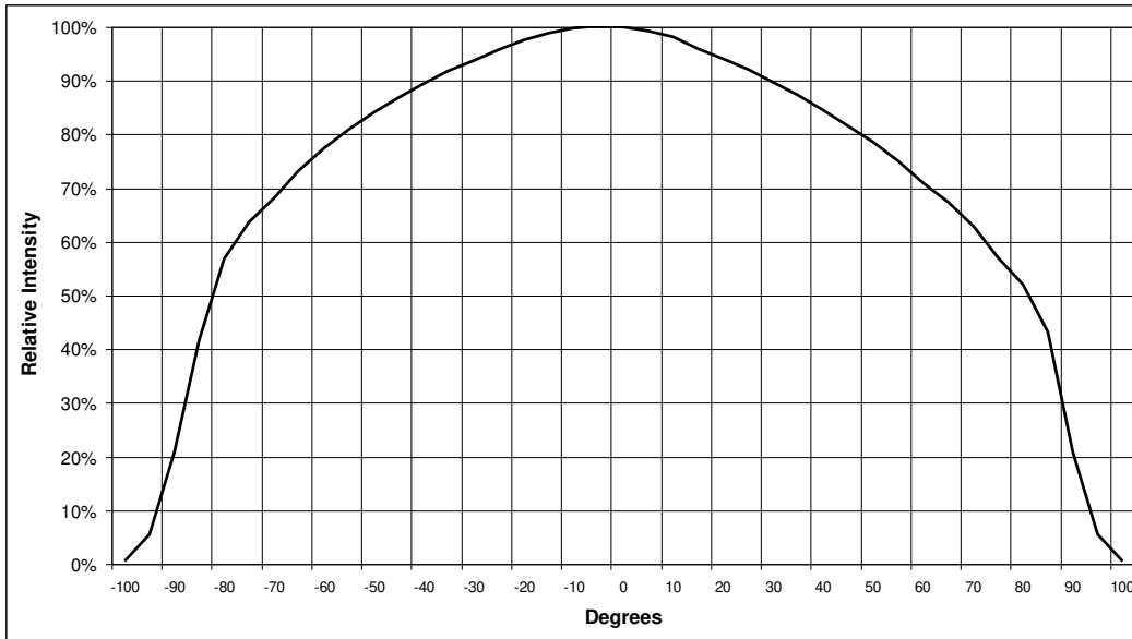
Figure 4: Typical Far Field Radiation Pattern
