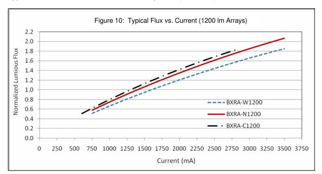
Typical Relative Luminous Flux vs. Current, T<sub>j</sub>=25° C (continued)
