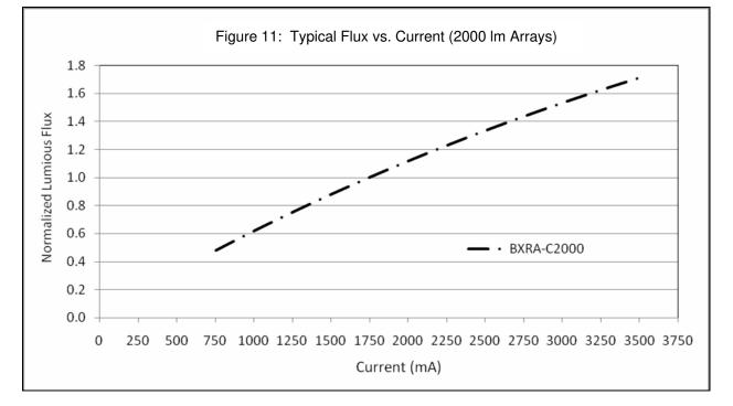
Note for Figures 8, 9, 10 and 11: Bridgelux does not recommend driving high power array devices at low currents. Doing so may produce unpredictable results. Pulse width modulation (PWM) is recommended for dimming effects.
