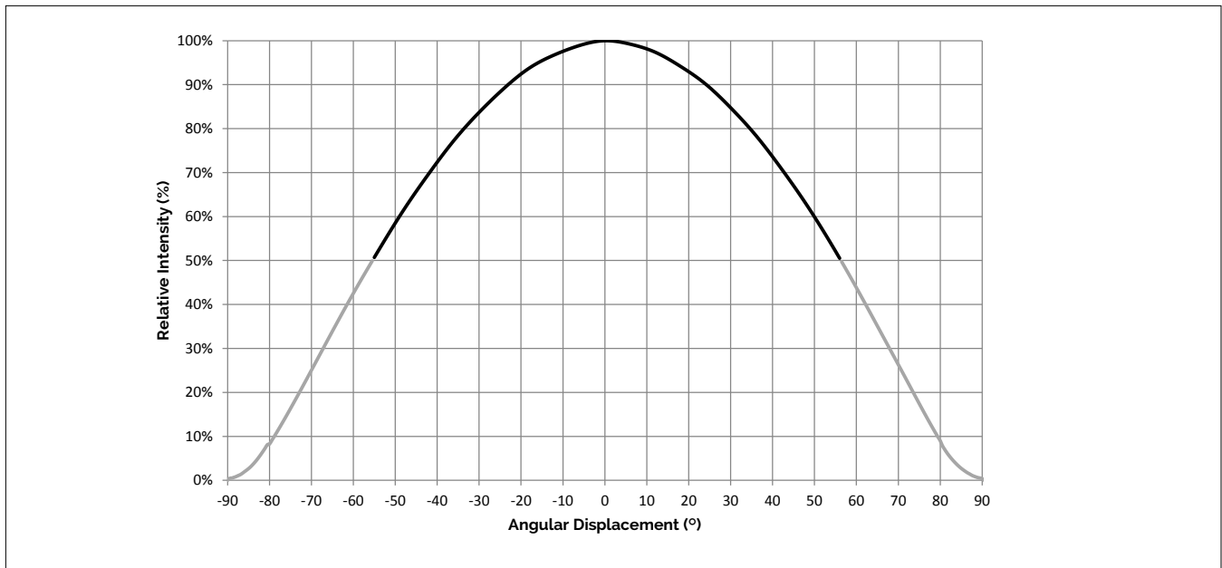
Figure 10: Typical Spatial Radiation Pattern
