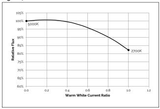
Figure 8: Derating Curve
