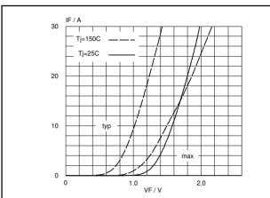
Fig.5. BY359X-1500 forward characteristic  $I_F = f(V_F)$ ; parameter  $T_j$
