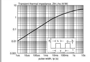
Fig.4. Transient thermal impedance  $Z_{th} = f(t_p)$
