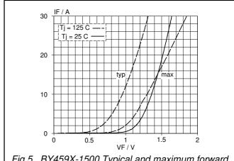
Fig.5. BY459X-1500 Typical and maximum forward characteristic  $I_F = f(V_F)$ ; parameter  $T_j$
