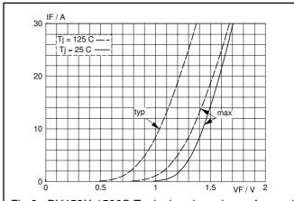
Fig.6. BY459X-1500S Typical and maximum forward characteristic  $I_F = f(V_F)$ ; parameter  $T_j$
