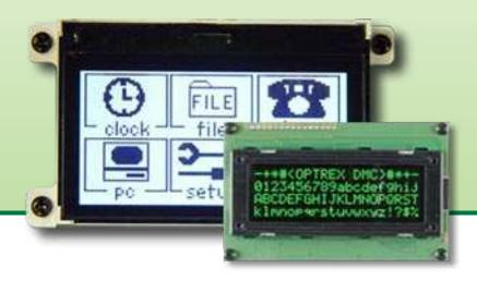
These new STN LCDs offer designers a range of passive matrix display solutions. Optrex STEP products deliver remarkable readability in any ambient lighting condition, with exceptional performance over a wide operating temperature range.
