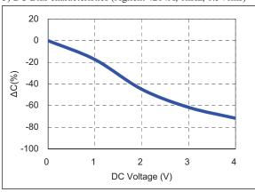
4) Bias TCC characteristics (Agilent 4284A, 1kHz, 0.5Vrms, 2Vdc)
