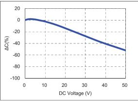
4) Bias TCC characteristics (Agilent 4284A, 1kHz, 1Vrms, 25Vdc)
