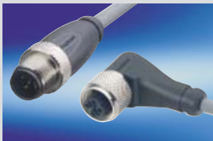
Cordset, unshielded Male connector, straight / Female connector, right angled with anti-vibration coupling nut A-coded
