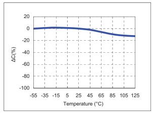
4) Bias TCC characteristics (Agilent 4284A, 1kHz, 1Vrms, 8Vdc)
