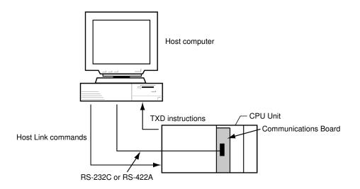
**Note** The RP Host Link command can be used for C200HX//HE/HE-CPU -ZE CPU Units only when a V1 Communications Board is mounted.
