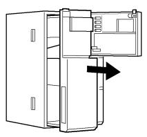
3. Slide in the Communications Board in slit and press it all the way to the back.
