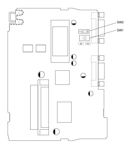
The factory settings are as follows. DIP switch SW1: 2 (2-wire) DIP switch SW2: 1 (Terminator OFF)
