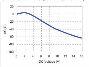
4) Bias TCC characteristics (Agilent 4284A, 1kHz, 1Vrms, 8Vdc)
