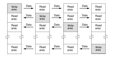
What determines what part of the LR area is allocated to which PC is the unit number assigned to each PC Link Unit. These numbers in turn determine which PC Link Units are **polling units** and which are **polled units**.
