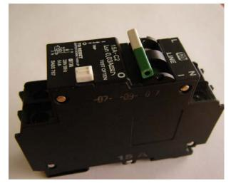
CE Approved UL 1077 and UL1053 recognized Sensitivity : 30 ma (CE) 22 ma (UL) Poles : 1 + N Voltage: 230 (CE) 240 (UL) Interrupting Rating : 5 KA Operation : Magnetic / Hydraulic – unaffected by ambient temperature Width : 26mm Weight : 0.57 lbs.
