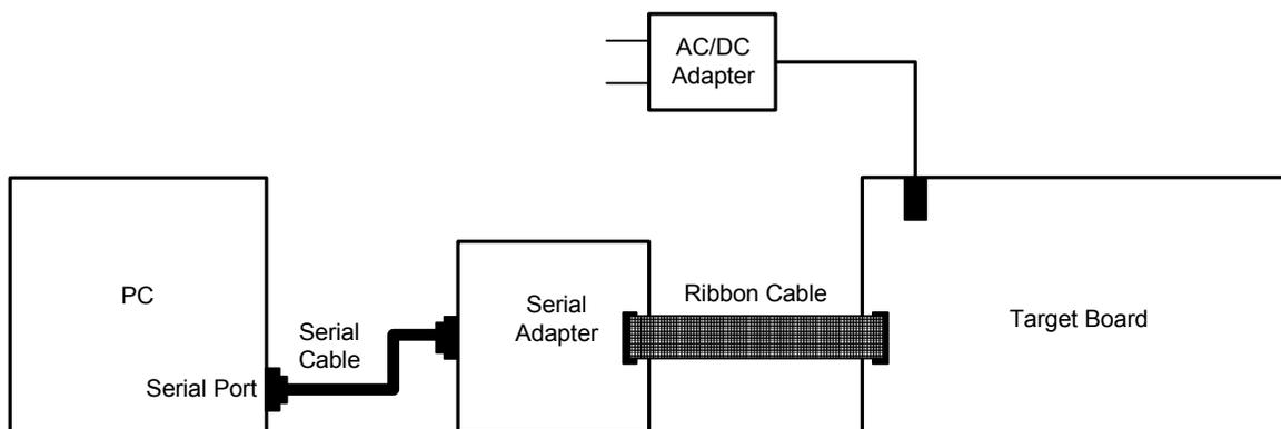
**Figure 1. Hardware Setup**
