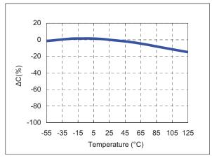
4) Bias TCC characteristics (Agilent 4284A, 1kHz, 1Vrms, 5Vdc)
