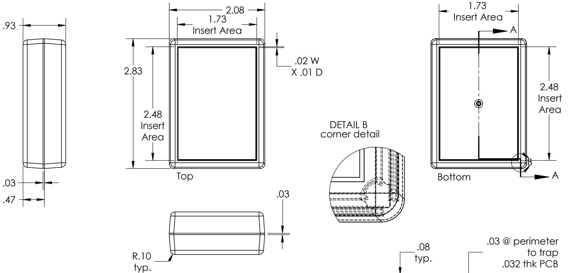
Enclosure can hold either a 0.032" PCB or a 0.063 PCB
