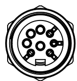
AISG 8-pin female interface with 4 loaded contacts
