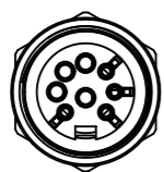
AISG 8-pin female interface with 4 loaded contacts
