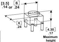
1.18 29 -Coin battery holder-location A .56 .55-.07¬ 0-1.86 .19 R.07 2 plc's 0 0. 0 0 Coin battery
